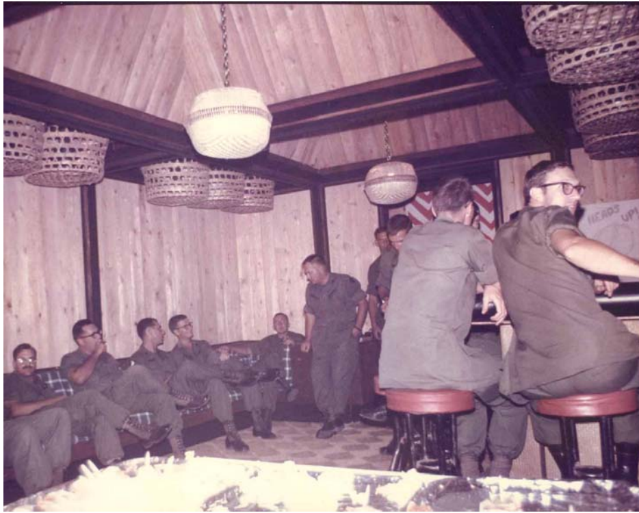
The HHC 159 th Officers Club designed by Tom Butt per orders of Col. Bratton. All materials were locally obtained. Some lights are made from bamboo baskets, others (downlights) from artillery casings. The “carpet” is woven grass. Carpentry was by Vietnamese carpenters working in the 92 nd Engineer Battalion Carpentry Shop. The only materials that did not come from local sources were the fabrics, which I picked up in Sydney, Australia. Col. Bratton went on to become a lieutenant general and Chief of Engineers in 1980.
